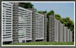
Built from 38x25 RHS frames, 50x10 RHS slats. Choose from a 20mm spacing or a 50mm spacing between slats as a standard range. Custom size spacing is also available. Over 100 powder coat colours to choose from.
